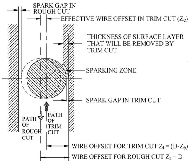
Figure 1 Details of trim cutting operation.
